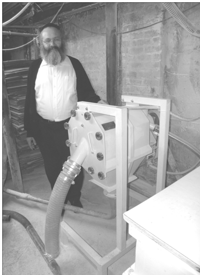
Mr. Weiss at the sifter. All flour travels by pipes.
